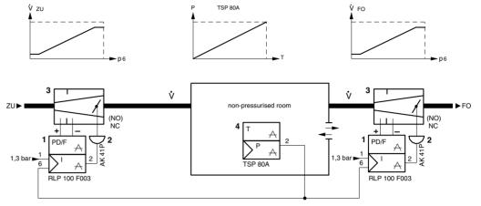
1. Control facility for variable volume flow without reheater for open rooms.
