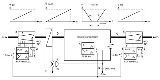
5. Control facility for variable volume flow with reheater for open rooms, reheater normally open, room temperature controller direction of action A
