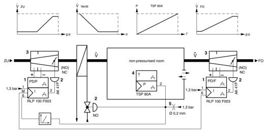
6. Control facility for variable volume flow with reheater for open rooms, reheater normally closed, room temperature controller direction of action B
