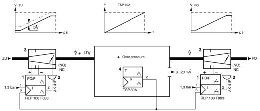
3. Control facility for variable volume flow without reheater for open rooms with negative pressure.
