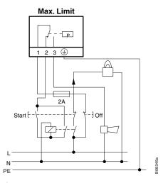
Pressure monitor as safety pressure limiter for falling pressure
